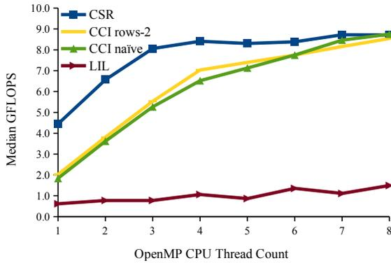
Figure 2: Multicore CPU scalability by data layout.
