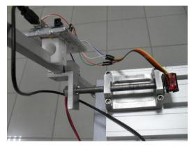
Fig. 2. Accelerometer location
