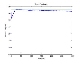
Fig. 5. Control results with gyroscope feedback alone
