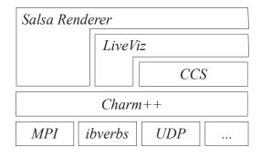
FIGURE 7.1: Software layer diagram for Salsa server-side renderer.
