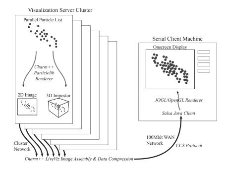
FIGURE 7.2: Data movement in Salsa. Particles are distributed across the cluster, rendered to 2D image or 3D impostor fragments, composited across the cluster, compressed and sent across the network to the client.
