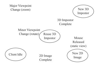
FIGURE 7.3: Finite state machine for network communication on the client.
