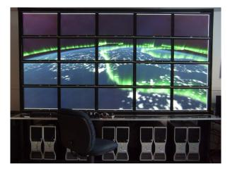
Figure 12: Interactive aurora rendering on a powerwall cluster with ten GPUs and twenty screens at 29fps.
