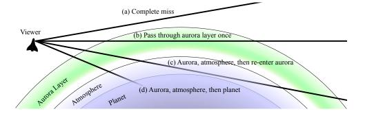
Figure 8: Possible ray/geometry intersection paths for camera rays originating outside the atmosphere.
