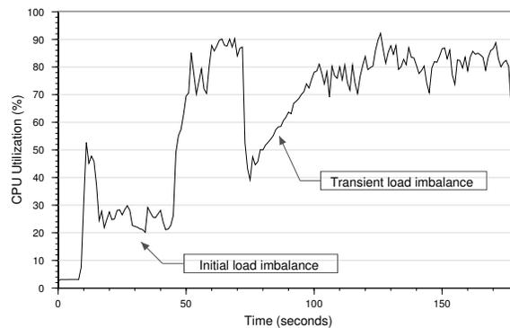
**FIGURE 9.8:** CPU utilization graph without load balancing (Tungsten Xeon).
