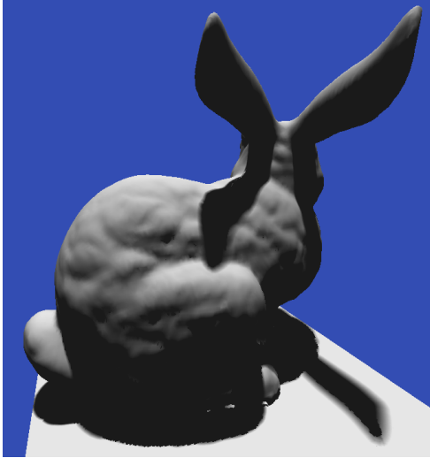
Figure 8. Stanford Bunny rendered using a 256x256 RGBA8 Penumbra Limit Map generated entirely on graphics hardware. Note self-shadowing errors at shadow of tip of right ear and base, and silhouette leakage at shadow of base of left ear.
