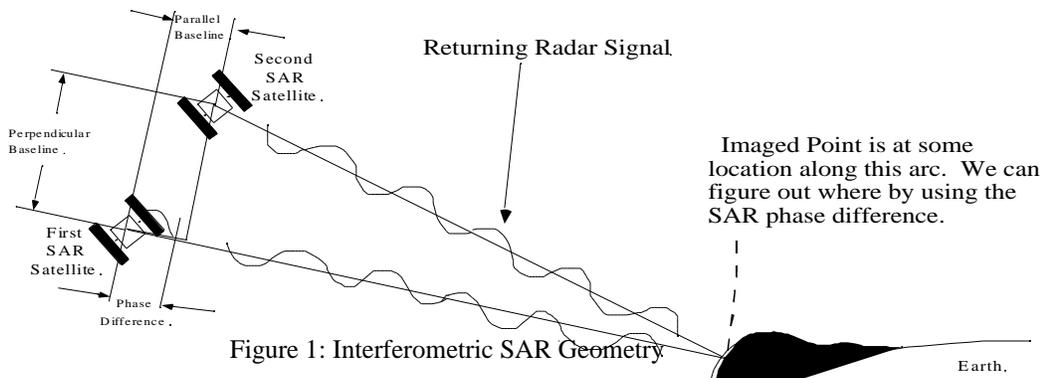
Figure 1: Interferometric SAR Geometry
