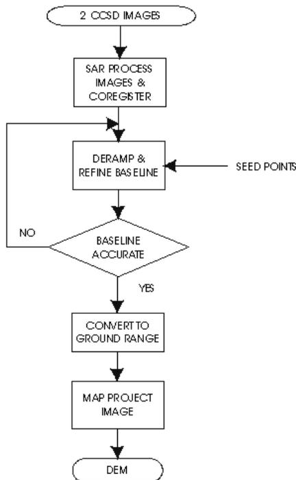
Figure 2: Software Flow Diagram
