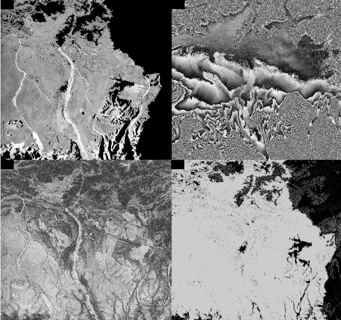
Figure 3A: Tie point locations 3B: phase image 3C: phase coherence image 3D: phase unwrapping mask
